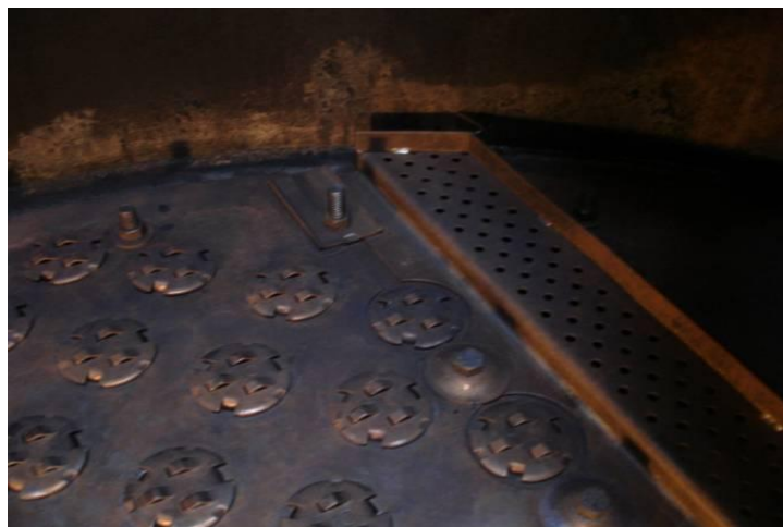
Figure 10 Advanced Dispersion Valve Tray with bubbling promoter
