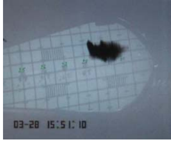
Fig. 11 pellet penetration measurement with image by ccd camera.
