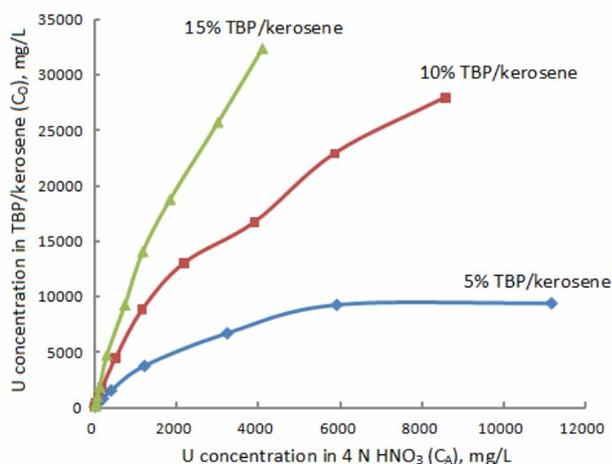
Fig. 1 Equilibrium distribution of uranium in 4 N  $HNO_3$  and TBP/kerosene.
