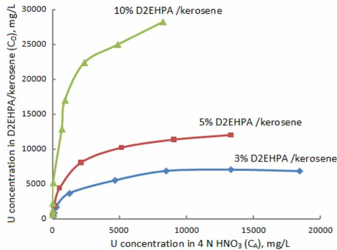
Fig. 2 Equilibrium distribution of uranium in 4 N HNO<sub>3</sub> and D2EHPA/kerosene.
