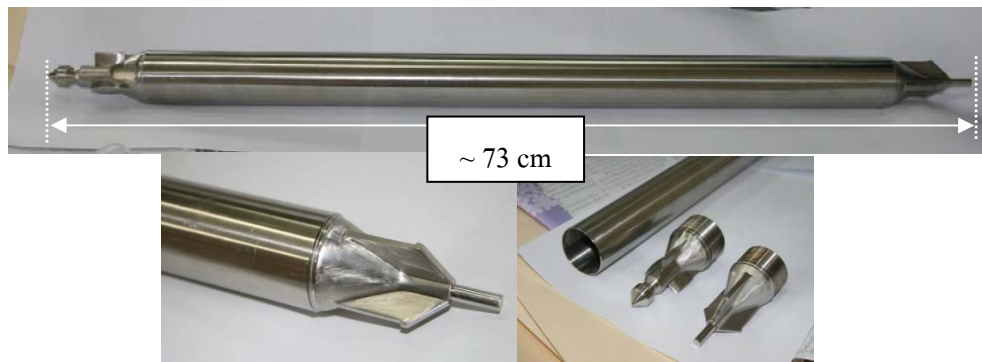
Fig. 2 Successfully fabricated mock up of the TRIGA research reactor fuel rod
