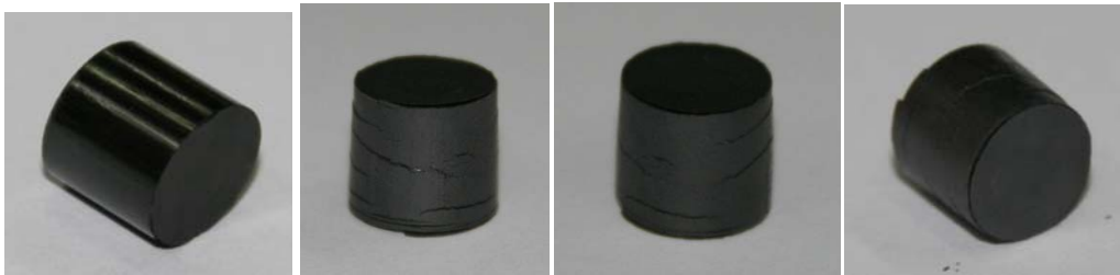
Fig. 5 Uranium oxide pellet after it was compressed (left) and sintered (three on the right).
