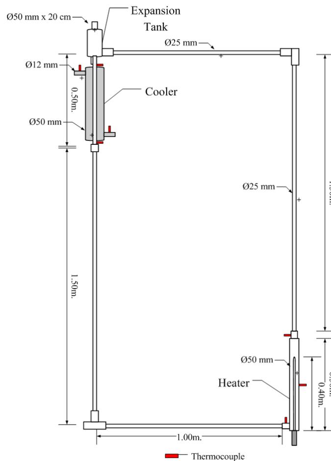
Fig. 1. Schematic of the rectangular natural circulation loop.
