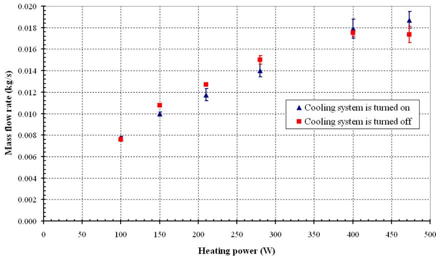
Fig. 4. Effect of heating power on the mass flow rates.
