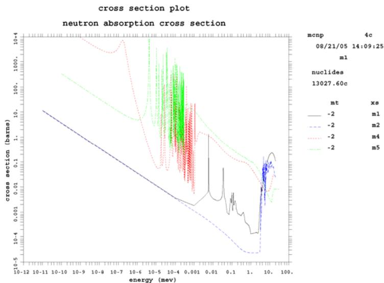
Figure 3: Comparisons of neutron absorption cross sections in different materials.
