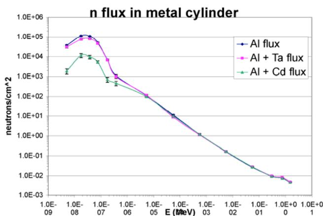
Figure 6: Neutron flux inside different kinds of metal tubes.
