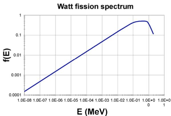
Figure 4: Watt fission energy distribution.
