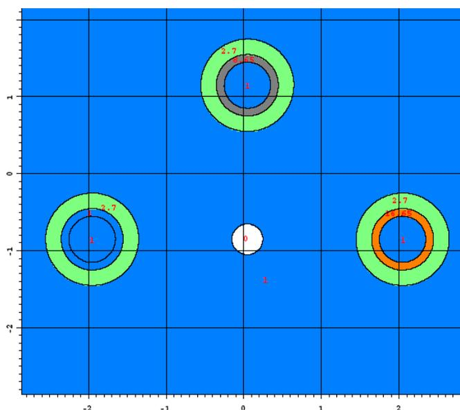
Figure 1: Top-view geometry of the setup. We have the neutron source in the middle and three cylindrical containers at equal distances from the source.
