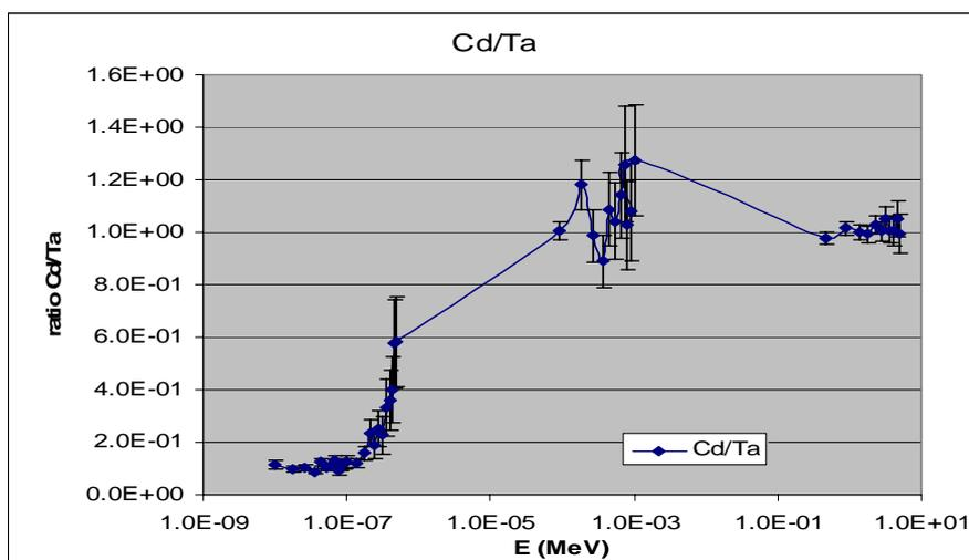
Figure 8: Ratio of neutron doses inside Cd/Al and Ta/Al containers.
